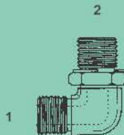
BPP-OFS-6801-NWO - Str. (1) Male O Ring Face Seal (SAE) (2) Male BPP Adj. O Ring w/ Retainer Washer
