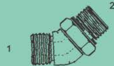
BPP-OFS-6802-NWO - 45° (1) Male O Ring Face Seal (SAE) (2) Male BPP Adj. O Ring w/ Retainer Washer
