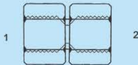
SS-MFL-6565-H - Str. (1) (2) Fem. Flareless Swivel Heavy
