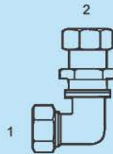
SS-MFL-2701-LN - Str. (1) Male Flareless (2) Male Flareless Bulkhead w/ Lock Nut Light
