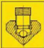
Ball thrust bearing in flaring cone minimizes friction, makes operation easier.
